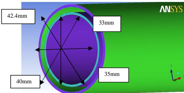
**Figure 2:** Dimensions of the heat exchanger
