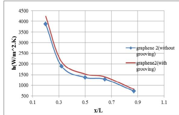
**Figure 12:** Heat transfer coefficient  $h$  ( $W/m^2.K$ ) with  $(x/L)$  for graphene2
