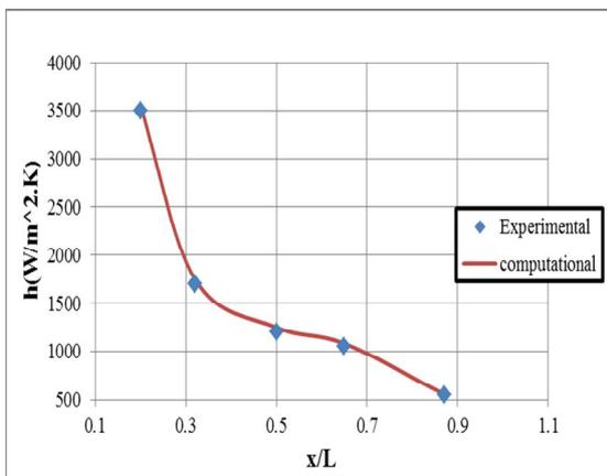
**Figure 6:** Heat transfer coefficient h (W/m<sup>2</sup>.K) with (x/L) for water.
