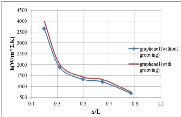
**Figure 9:** Heat transfer coefficient  $h$  ( $W/m^2.K$ ) with  $(x/L)$  for graphene1
