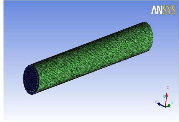
**Figure 4:** Meshing of double tube heat exchanger
